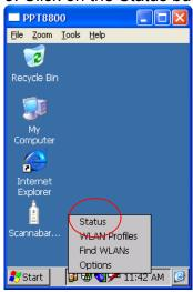
4. In the screen that opens you will be able to verify your Signal Strength under the signal tab.
